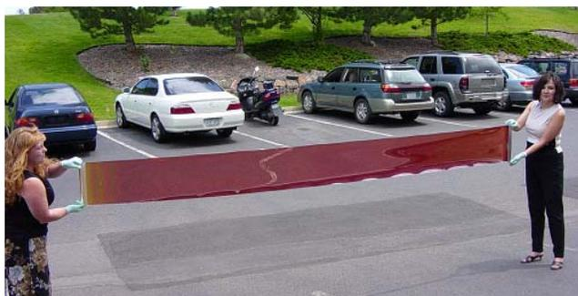
Amorphous silicon deposited on plastic in a reel to reel cassette cluster tool system- 30cm web width.
